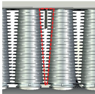
Figure 2.5 Air passage between 2 Robur exchangers
