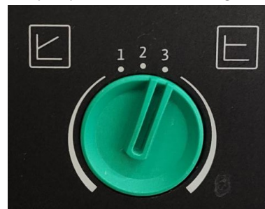
Figure 1.33 AY pump selector switch setting
